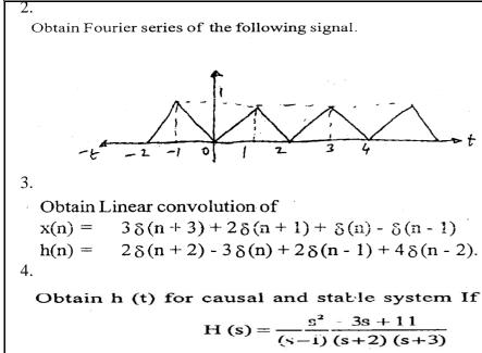
Plot the ROC and pole's and zero's of the system.
